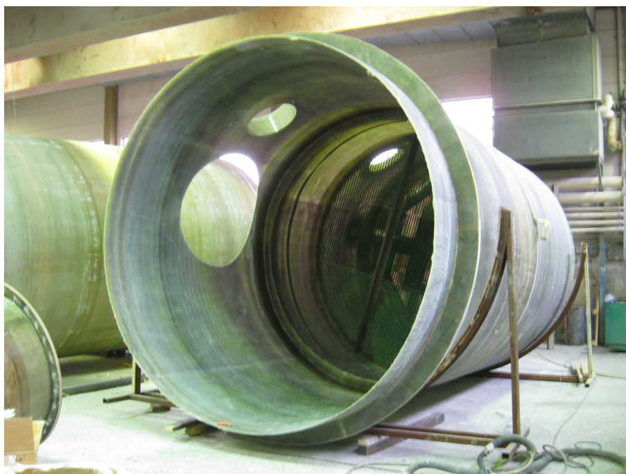
Figure – Manufacturing of scrubber tower for Västervik Miljö & Energi AB.
