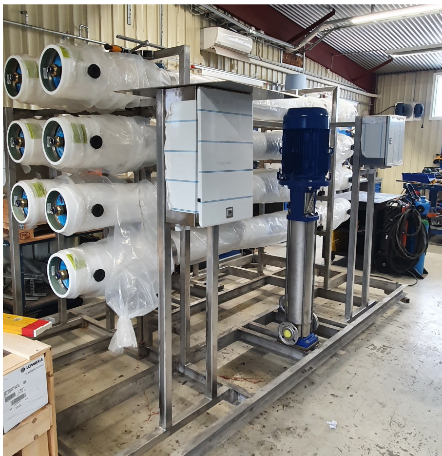
Figure – Manufacturing of Reverse osmosis skid.
