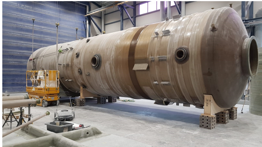
Figure – Manufacturing of scrubber tower.
